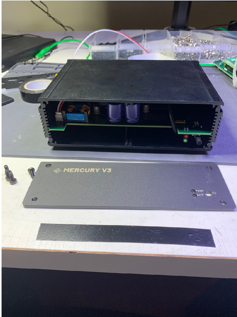
Figure 6 – Step 1, Remove Front Panel Screws
