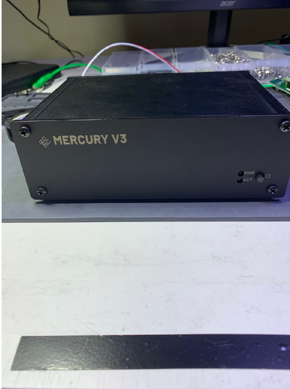
Figure 10 – Step 5, screw the front panel back into place
